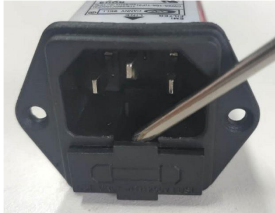
Figure 6. 1 Use a tool to push out the power socket
