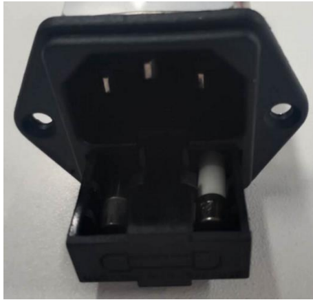
Figure 6. 3 Make the new fuse lay flat in the drawer.
