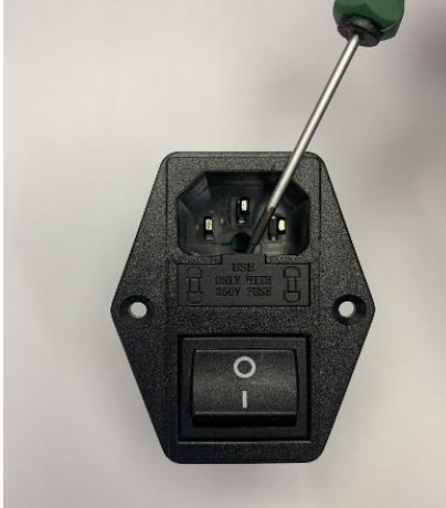
Figure 6. 1 Use a tool to push out the power socket
