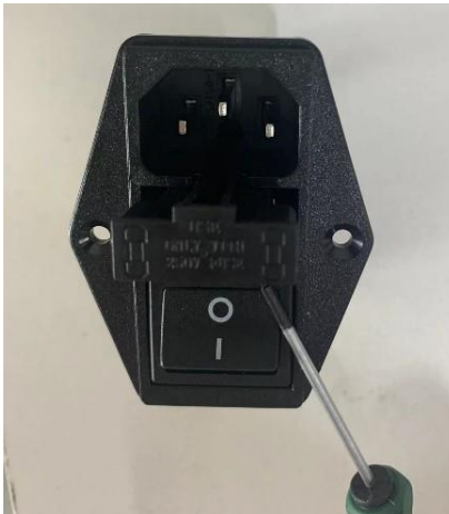
Figure 6. 2 Use a tool to gently lift the fuse
